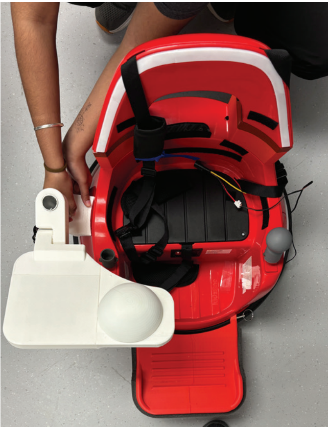
Image 3: A button cover to prevent accidental actuation.
