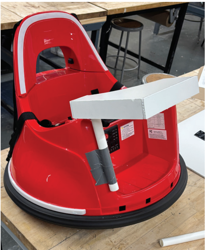
Image 4: First mock-up of the tray, demonstrating size and scale and iteration with user.
