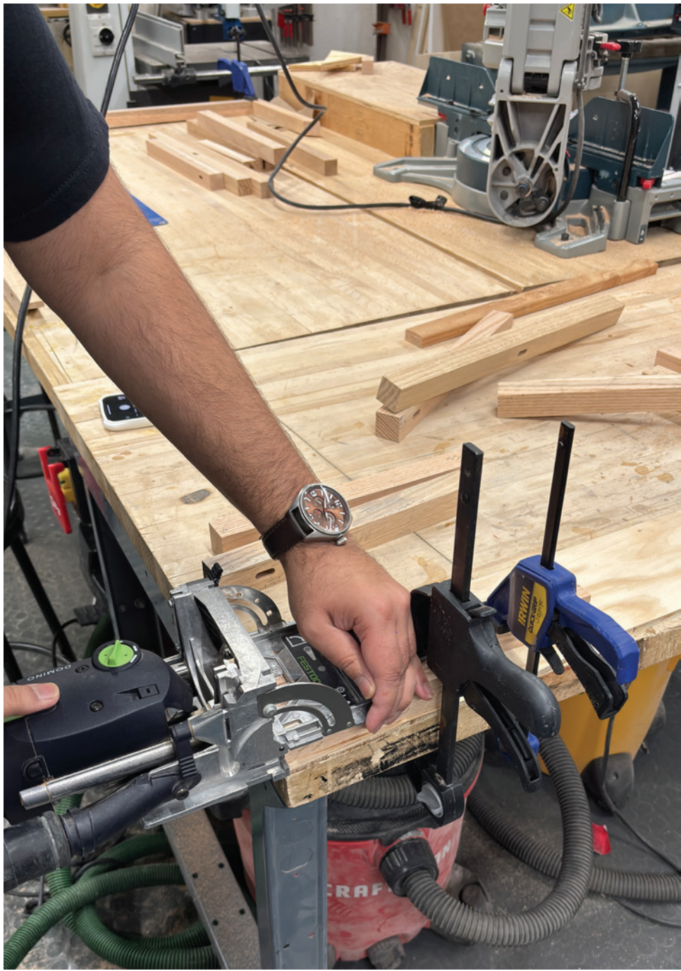
Image 1: Using domino joiner to make joins
