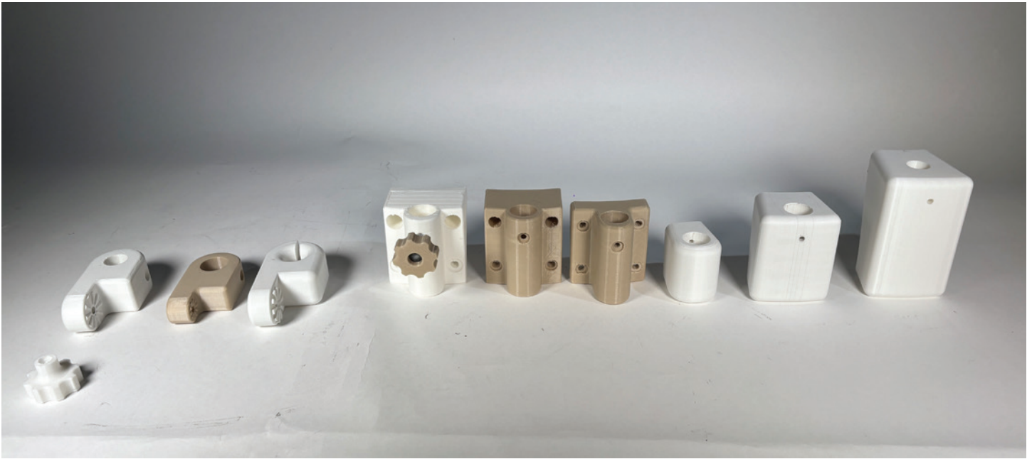
Image 3: All the iterations of the parts, the mount for pipe, the knob for tightening the articulation points
