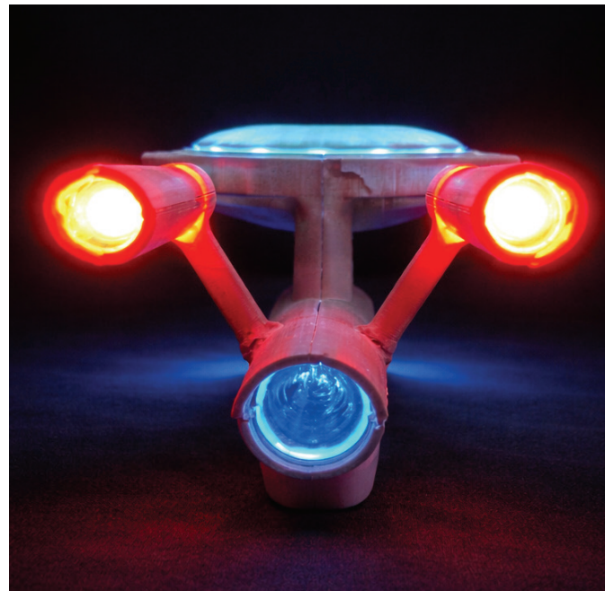
Image 3: A view showing light-pipes in action
