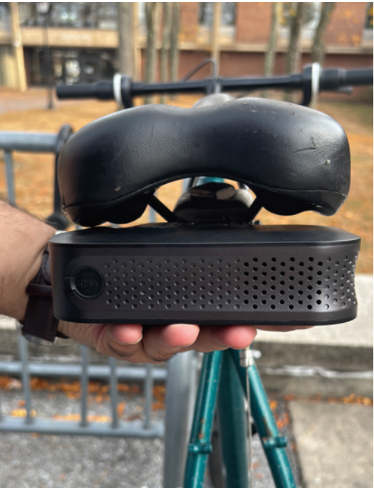
Image 2&3: Possible mounting orientations for the inflator beneath the saddle via the bike rail mount.
