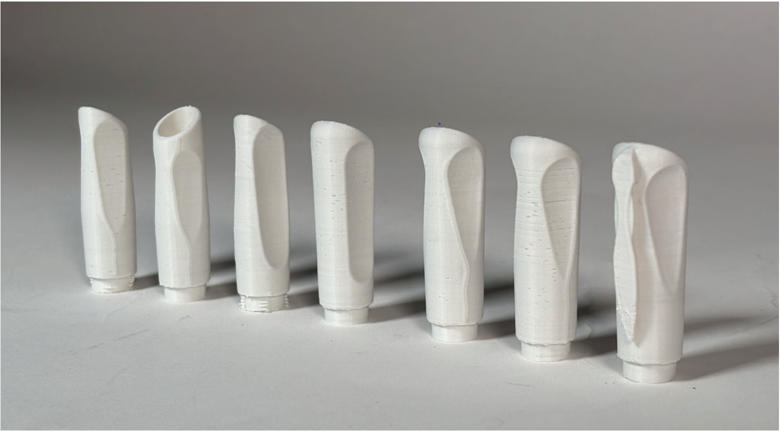
Image 1: Grip Refinement models for User validation. Starting from Left and final one on right.
