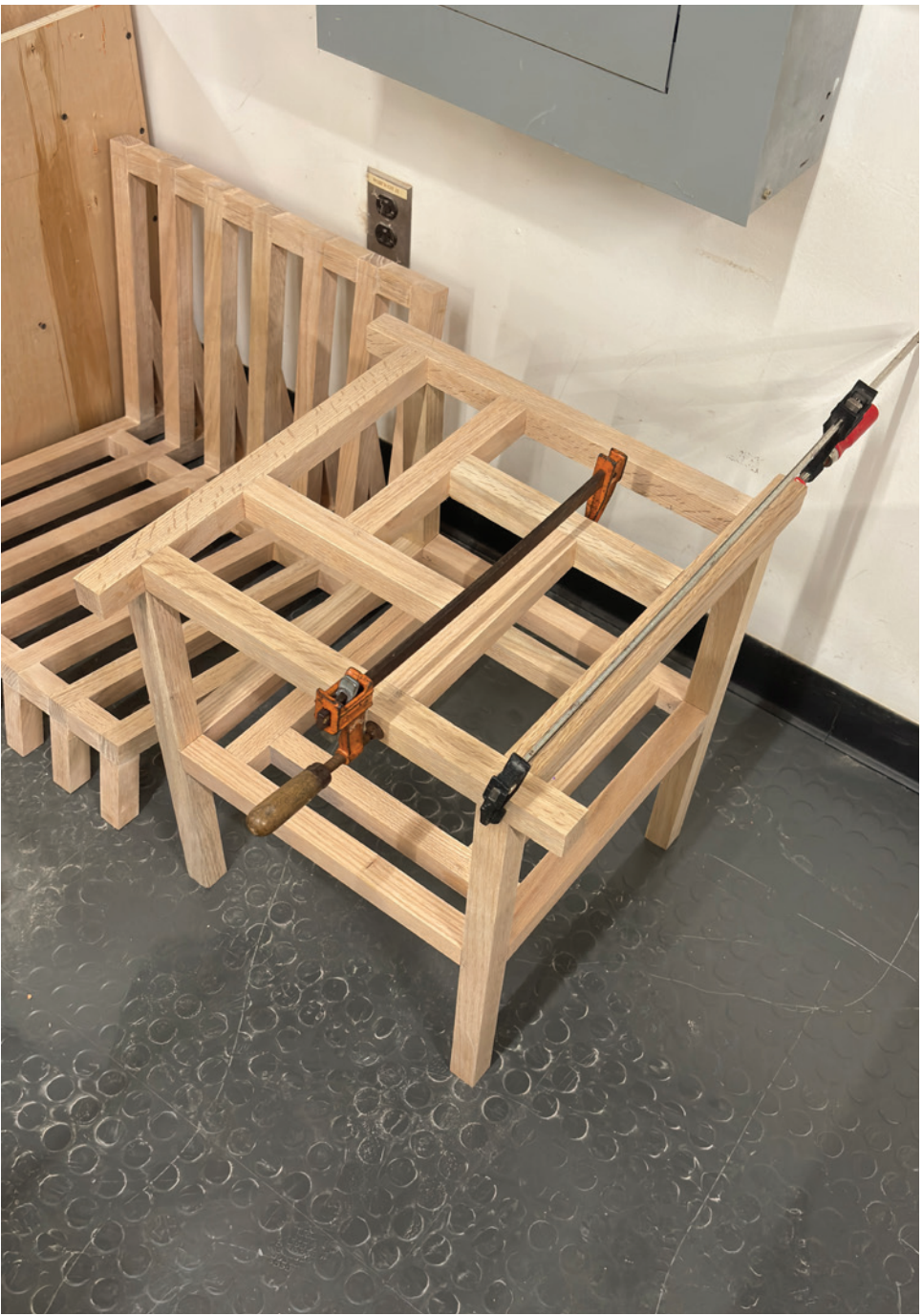
Image 3: Pre-Final assembly to check how is everything fitting.
