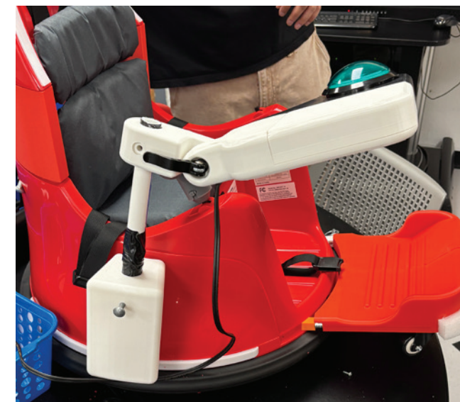
Image 2: Prototype 1.0 on tray, sagging due it being heavy.
